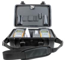
Using the power meter with an optical light source enables the engineer to measure the optical loss in fibre optical cables.
