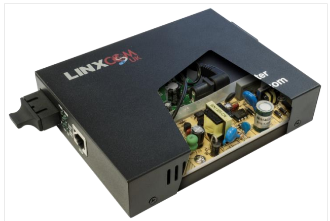
Internal power Supply
