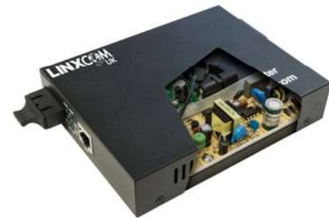
INTERNAL POWER SUPPLY
